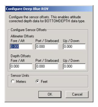
In this dialog box enter the offsets from the CRP of the ROV to the sensor locations. Fore/Aft offsets are entered similar to all devices in WinFrog with Forward/Starboard offsets being positive and Aft/Port offsets being negative. The Up/Down offsets are vertical offsets with Up being positive and Down being negative. The units output by the sensors have to be selected as either meters or feet.
